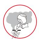
Keep your head out of the fumes. Do not breathe the fumes. Use enough ventilation, exhaust at the arc, or both, to keep fumes and gases from your breathing zone and the general area. The recommended way to determine adequate ventilation is to sample for the composition and quantity of fumes and gases to which personnel are exposed.
