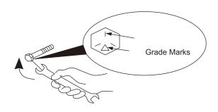
If necessary, always replace any fastener with one of equal size, grade, and type.
