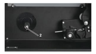
**Note:** a slight drag is necessary and should be provided correctly by the spool retainer spring. The drag will prevent the wire from continuing to spin and unwind itself each time you release your torch trigger. Should the drag be too tight, you may have to remove the sticker from your wire spool to provide more movement room.
