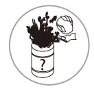
Do not weld on containers that have held combustibles, or on closed containers such as tanks, drums, or pipes unless they are properly prepared according to AWS F4.1 and AWS A6.0 (see Safety Standards in Section 9).
