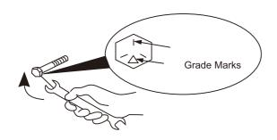
If necessary, always replace any fastener with one of equal size, grade, and type.
