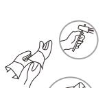
Wear dry, hole-free insulating gloves and body protection. Do not touch electrode with bare hand. Do not wear wet or damaged gloves.
